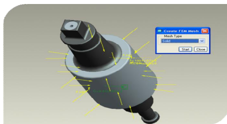
Fig. 6 Mathematical Model of Roll with Forces and other properties in Dynamic Module Analysis.
